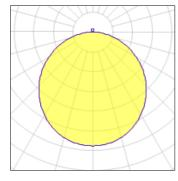
Lamp type LED CCT 3000 K Nominal lamp power 24 W CRI 80 Total flux LOR 100% 2530 lm Luminous efficacy 105 lm/W ULOR 2% Total power 24 W
