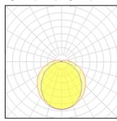
Lamp type Nominal lamp power Total flux Luminous efficacy LED 60 W 8900 lm 148 lm/W CCT
