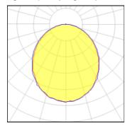
LED CCT 4032 K Lamp type Nominal lamp power 21.08 W CRI 80 Total flux 2454 lm LOR 100% 116 lm/W 21.08 W Luminous efficacy Total power
