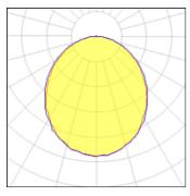
CCT Lamp type LED 4032 K Nominal lamp power 21.08 W CRI 80 Total flux 2454 lm LOR 100% Luminous efficacy 116 lm/W Total power 21.08 W
