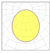
CCT 4032 K Lamp type LED Nominal lamp power 21.08 W CRI 80 100% 2454 lm Total flux LOR Luminous efficacy 116 lm/W Total power 21.08 W
