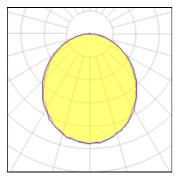
4032 K Lamp type LED CCT Nominal lamp power 21.08 W CRI 80 Total flux 2454 lm LOR 100% Luminous efficacy 116 lm/W 21.08 W Total power
