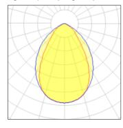
Lamp type Nominal lamp power Total flux Luminous efficacy LED 41 W 4465 lm 109 lm/W CCT
