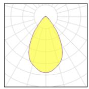
1 x LED Nominal lamp power 72 W LOR 85% Lamp flux 8460 lm Total flux 7158 lm Luminous efficacy 118 lm/W Total power 80 W CCT 3000 K CRI 80
