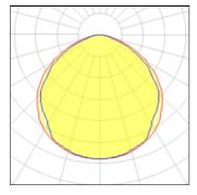
Lamp type Nominal lamp power Total flux Luminous efficacy LED 600 W 78000 lm 130 lm/W CCT CRI LOR Total power 5000 K 70 100% 600 W
