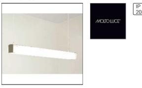
Messina, Hanging lamp made of extruded, anodized aluminum; end caps anodized aluminum; Side Cover of white satin acrylic; homogeneous, shadow-free light, Light emission by all sides; height adjustable without tools, injection transparent, 3x1mm <sup>2</sup>; Opal diffuser to prevent glare; IP 20;
