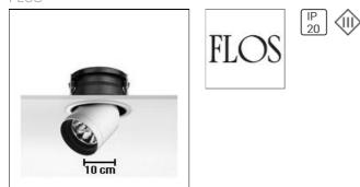
Recessed luminaire for indoor application. For very low voltage halogen lamps or standard and discharge lamps. Self-extinguishing ceramic or engineering plastic lamp holders, with single-pole, transparent electric wires with double Teflon insulation.
