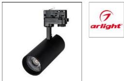
Hanging light for tracks/buses 4 wires for products. Power 20 W, luminous flux 1700 lm, 85 lm/W, special cold 7500 K for fish and seafood, angle 24°, supply voltage 230 V. Black aluminum housing, PMMA lens material, protection degree IP20. Size: diameter 74 mm, height 160 mm. Installation on a 3-phase track. Driver 30-42 V, 500 mA, ripple <1%.
