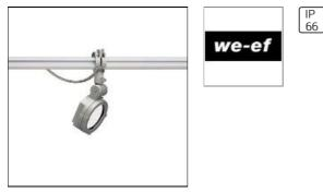
IP66, Class I. IK07. Marine-grade die-cast aluminium alloy. 5CE superior corrosion protection including PCS hardware. Silicone rubber gaskets. Safety glass lens. PMMA-LED lens array. Including 0,4 m of flexible cable enclosed in stainless conduit, in-line connector and mounting clamp for installation to RAIL66 mounting system.
