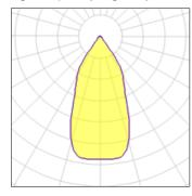
Lamp type Nominal lamp power Total flux Luminous efficacy LED 19 W 2051 lm 108 lm/W CCT
