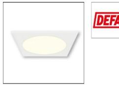
Interior fitting to be recessed in T-profile ceiling. Frame in aluminium powder painted in white RAL 9010. Opal acrylic diffuser. Ledge is delivered "plug&play", complete with 1.5m 2-pol cable and plug from driver. DALI version supplied with 1.5m 4pol cable from driver, DALI entries with DA, DA marking. The driver and the LED panel are connected with 1m cable.
