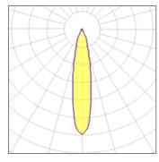
CCT 4000 K Lamp type LED Nominal lamp power 2.75 W CRI 90 Total flux 215 lm LOR 100% Luminous efficacy 78 lm/W Total power 2.75 W
