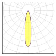
4000 K Lamp type LED CCT Nominal lamp power 2.75 W CRI 90 Total flux 215 lm LOR 100% Luminous efficacy 78 lm/W Total power 2.75 W
