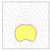
CCT 3000 K Lamp type LED Nominal lamp power 28 W CRI 80 LOR 100% Total flux 1454 lm Luminous efficacy 52 lm/W ULOR 10% Total power 28 W
