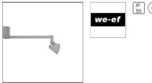
IP55, Class I. Marine-grade die-cast aluminium alloy except outreach arm which is extruded. 5CE superior corrosion protection including PCS hardware. Silicone CCG® Controlled Compression Gasket. Safety glass lens, hinged. Anodised aluminium reflector. Two cable entries. Knuckle permits 350° horizontal and 90° vertical aiming of optics.
