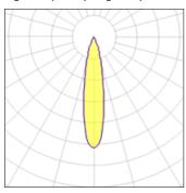
CCT 2700 K Lamp type LED Nominal lamp power 2.75 W CRI 90 Total flux 186 lm LOR 100% Luminous efficacy 68 lm/W Total power 2.75 W
