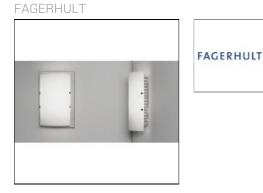
Installation Luminaire for wall installation. Two fixing holes. Connection Snap-in terminal block 3x2.5 mm<sup>2</sup> or 5x2.5 mm<sup>2</sup> when dimming. LED luminaire connects via 230 V, built-in LED driver. 1-phase through-wiring possible. Surface mounted mains cable possible. Design Luminaire body and rear section of alu-grey sheet steel. Diffuser of opal matt glass. Alu-grey (RAL 9006) structured rear plate. Integrated HF-ballast. Dimming DALI/Phase-pulse control as standard.
