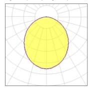
Lamp type LED CCT 3000 K Nominal lamp power 22 W CRI 80 Total flux LOR 100% 2300 lm Luminous efficacy 105 lm/W Total power 22 W
