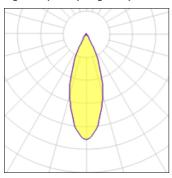
CCT 2700 K Lamp type LED Nominal lamp power 2.75 W CRI 90 Total flux 174 lm LOR 100% Luminous efficacy 63 lm/W Total power 2.75 W
