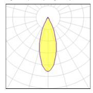
LED CCT 2700 K Lamp type Nominal lamp power 2.75 W CRI 90 Total flux 174 lm LOR 100% 63 lm/W 2.75 W Luminous efficacy Total power
