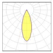
2700 K Lamp type LED CCT Nominal lamp power 2.75 W CRI 90 Total flux 174 lm LOR 100% Luminous efficacy 63 lm/W Total power 2.75 W
