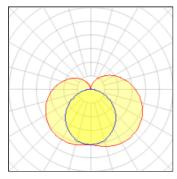
CCT 2700 K Lamp type LED Nominal lamp power 16 W CRI 90 LOR 100% Total flux 900 lm Luminous efficacy 56 lm/W ULOR 24% Total power 16 W
