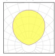
Lamp type LED CCT 2962 K Nominal lamp power 1 W CRI 80 Total flux 100% 10 lm LOR Luminous efficacy 10 lm/W ULOR 100% Total power 1 W
