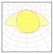
1 x Metal halide lampKetal halide lampNominal lamp power70 WLORLamp flux7200 lmTotal fluxLuminous efficacy63 lm/WTotal powerCCT3000 KCRI9090CRI
