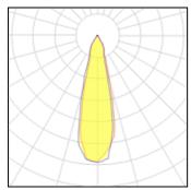
1 x LED Nominal lamp power 12 W LOR 68% Lamp flux 1660 lm Total flux 1136 lm Luminous efficacy 138 lm/W Total power 15 W CCT 4000 K CRI 80
