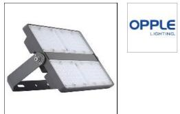
Housing: PC Mounting ring: Grey; Installation: Bracket; Dimensions: 376\*288\*59mm Power: 200W; Efficacy: 96 Lm/w Colour temperature: 4000K; Colour rendering: RA80; Total luminous flux of luminaire: 19200Lm Beam angle:70+28° Service life: 30,000h Degree of protection: IP65; Class of protection Mains voltage: 220-240V/50-60Hz;
