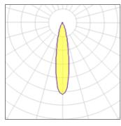
CCT 2700 K Lamp type LED Nominal lamp power 2.75 W CRI 90 Total flux 189 lm LOR 100% Luminous efficacy 69 lm/W Total power 2.75 W
