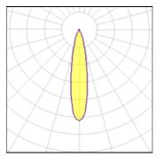
2700 K Lamp type LED CCT Nominal lamp power 2.75 W CRI 90 Total flux 189 lm LOR 100% Luminous efficacy 69 lm/W Total power 2.75 W
