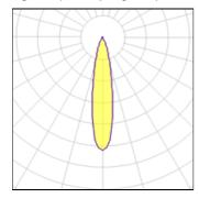
LED CCT 2700 K Lamp type Nominal lamp power 2.75 W CRI 90 Total flux 189 lm LOR 100% 69 lm/W 2.75 W Luminous efficacy Total power
