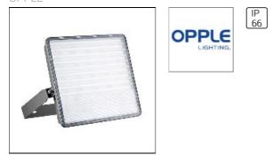
Housing: Die-cast Aluminum; Mounting ring: Grey; Installation: Bracket/ Pole; Dimensions: 352\*363\*54mm; Ceiling cutouts: /; Beam angle: 35°\*80°; Lamp(s): LED; Power: 200W; Efficacy : 95Lm/w Total luminous flux of luminaire: 20000lm; Power Factor: 0.95 Mains voltage: AC220-240V/50-60Hz; Colour temperature: 3000K; Colour rendering: Ra80; UGR: / IP/IK Grade: IP66/ IK06; Class of protection I; Control System: / Service life: 30,000h at 70% luminous flux;
