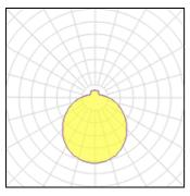
Lamp type LED CCT 4000 K Nominal lamp power 17 W CRI 80 Total flux 2110 lm LOR 100% Luminous efficacy 124 lm/W ULOR 17% Total power 17 W
