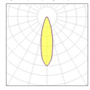
Lamp typeLEDCCTNominal lamp power4 WCRITotal flux158 lmLORLuminous efficacy40 lm/WTotal power
