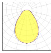
Lamp type Nominal lamp power Total flux Luminous efficacy LED 28 W 2900 lm 104 lm/W CCT
