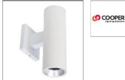
Distributions: 15°, 25°, 40° and 55°, Mounting: ceiling, wall or stem, Extruded aluminum housing; Die-cast or spun aluminum reflectors, 6 color temperatures: 2400K, 2700K, 3000K, 3500K, 4000K and 5000K CCT, CRI: 80, 90 or 97; D2W<sup>™</sup> option from 3000K to 1850K, Lumens: 500, 1,000 1,500 and 2,000, Colors: Matte Black, Matte White, Bronze and Silver paint finishes, Standard 0-10V dimming down to 1%, ENERGY STAR® qualified, 5-year warranty, Integral or remote driver options
