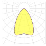
Lamp typeLEDCCTNominal lamp power0.8 WCRITotal flux1 lmLORLuminous efficacy1 lm/WTotal p
