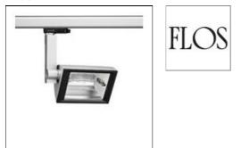
Range of indoor spotlights for accent and general lighting for three-phase track and wall/ceiling installation. Die-cast aluminium alloy, powdercoated optics compartment, diameter 118 mm, composed of an aluminium dissipating element placed above the lamp support, a black thermoplastic screen support ring and 4 mm tempered glass cover. Integrated auxiliary power units for the lamps inside a die-cast aluminium alloy container with powder-coated finish.
