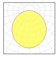
Lamp type Nominal lamp power Total flux Luminous efficacy LED 11.4 W 1365 lm 120 lm/W CCT
