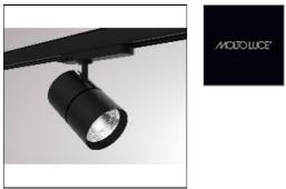
MOVA M BASIC TRACK TRACK SPOTLIGHT WITH 3 PH ADAPTER made of aluminium, black, similar to RAL 9005, decor black, high-efficiently vacuum deposited aluminium reflector without safety glass beam 17°, light output direct, swiveling 350, tilting 90, with converter, max. 800mA, dimmability: Pulse-DALI, adapter/ceiling base black, IP20
