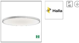
290-260K-10GHM3/830, W Luminaire surface/wall mounted/suspended Material of luminaire: Colour of luminaire: Shape of luminaire: Circular Size: 630 x 630 x 24 mm Type of installation: Surface, Wall mounted, Suspended Distribution: Direct Optics type: Opal diffuser Protection class: I Voltage: 220-240V
