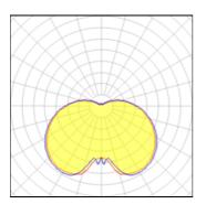
1 x Metal halide lamp Nominal lamp power 70 W Socket G12 Lamp flux 6600 lm LOR 8% Luminous efficacy 94 lm/W Total flux 518 lm CCT 3000 K Total power 83 W CRI 88
