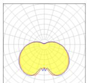
1 x Metal halide lamp Nominal lamp power 70 W Socket G12 Lamp flux LOR 6600 lm 8% Luminous efficacy 94 lm/W Total flux 518 lm CCT 4000 K Total power 83 W CRI 94
