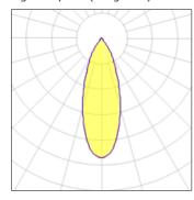
Lamp type LED CCT 4000 K Nominal lamp power 45 W CRI 90 Total flux 3600 lm LOR 100% Luminous efficacy 80 lm/W Total power 45 W
