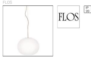
Ceiling mounted fixture providing dif-fused lighting. Diffuser consisting of an externally acid-etched, hand blown, flashed opaline glass. Gloss white pain-ted pressed steel diffuser support. 30% fiberglass reinforced injection-molded polyamide rose; pressed and galvanized ceiling fitting. Steel suspension cable, transparent FEP/PVC power cord, length 3700 mm. Net weight 2,7 kg.
