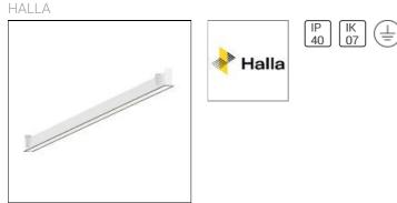
35-000K-25GGE/840, S Luminaire recessed Material of luminaire: Colour of luminaire: Shape of luminaire: Linear Size: 1423 x 54 x 95 mm Type of installation: Recessed Distribution: Direct Optics type: Opal diffuser Protection class: I Voltage: 220-240V
