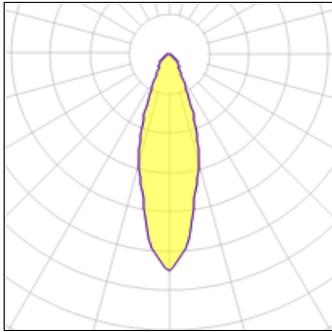
**1 x Halogen low voltage lamp without reflector**
