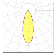
Lamp type LED CCT 3000 K Nominal lamp power 45 W CRI 90 Total flux LOR 100% 3375 lm Luminous efficacy 75 lm/W Total power 45 W
