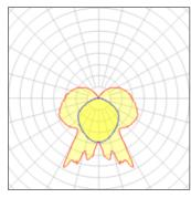
CCT 3000 K Lamp type LED Nominal lamp power 13 W CRI 80 LOR 100% Total flux 1250 lm Luminous efficacy 96 lm/W ULOR 23% Total power 13 W
