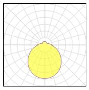
Lamp type LED CCT 3000 K Nominal lamp power 32 W CRI 80 Total flux 3880 lm LOR 100% Luminous efficacy 121 lm/W ULOR 15% Total power 32 W
