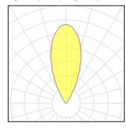
LED CCT 3783 K Lamp type Nominal lamp power 2.9 W CRI 80 Total flux 100% 299 lm LOR Luminous efficacy 103 lm/W ULOR 100% Total power 2.9 W
