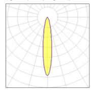
LED CCT 3000 K Lamp type Nominal lamp power 26 W CRI 80 Total flux 100% 1402 lm LOR Luminous efficacy 54 lm/W Total power 26 W
