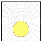
CCT 2700 K Lamp type LED Nominal lamp power 96 W CRI 90 69% Total flux 2628 lm LOR Luminous efficacy 27 lm/W Total power 96 W
