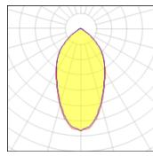
Lamp type Nominal lamp power Total flux Luminous efficacy LED 173.7 W 30000 lm 173 lm/W CCT
