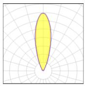
Lamp type LED CCT 4000 K Nominal lamp power 32 W CRI 80 Total flux 2135 lm LOR 100% Luminous efficacy 67 lm/W ULOR 100% Total power 32 W
