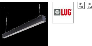
Suspended decorative luminaire for LED light sources; powder-coated aluminum profile equipped with an efficient lighting system, optimized for indoor use. Mounting: suspended, on wire suspension (on request) Body: aluminum profile Power supply efficiency: >87% Power: 220-240V 50/60Hz Includes light source: yes Lifetime (L80B10): 100 000 h Lifetime (L90B10): 50 000 h Warranty: 5 years Application: offices, hotels, reception desks, galleries, auditorium, boutiques, museums
