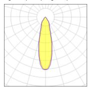
CCT Lamp type LED 4000 K Nominal lamp power 2.59 W CRI 90 Total flux 218 lm LOR 100% Luminous efficacy 84 lm/W Total power 2.59 W
