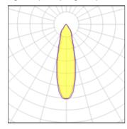
LED CCT 4000 K Lamp type Nominal lamp power 2.59 W CRI 90 Total flux 218 lm LOR 100% 84 lm/W 2.59 W Luminous efficacy Total power
