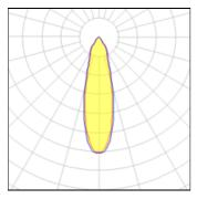
4000 K Lamp type LED CCT Nominal lamp power 2.59 W CRI 90 Total flux 218 lm LOR 100% Luminous efficacy 84 lm/W Total power 2.59 W
