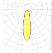
CCT 4000 K Lamp type LED Nominal lamp power 2.59 W CRI 90 Total flux 218 lm LOR 100% Luminous efficacy 84 lm/W Total power 2.59 W
